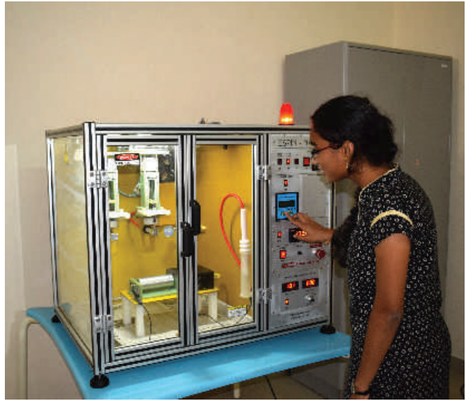
A student conducting experiment in Electro spinning Apparatus
