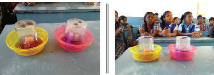
Rise of water in the tilted jar when the candle inside goes off
